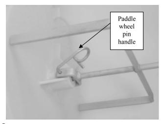
2 Un-clip the hand-removable paddle wheel pin from the agitator...
